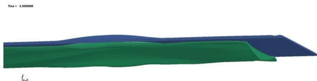
Figure 5 Hull and V-bottom plate deformation at 7 ms (left-bottom view)
