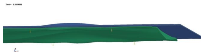
Figure 13 Hull and V-bottom deformation with bolts and their springs at 7 ms (left-bottom view)
